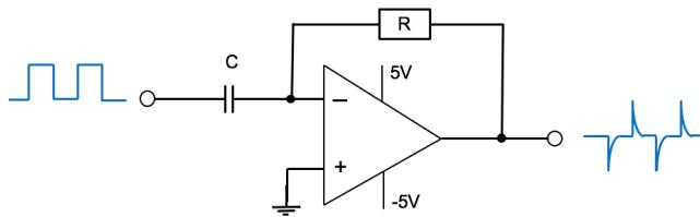
Swapping R and C in both passive and op-amp circuit for the two circuits as integrators yields two differentiator circuits. Both provide an approximation to the differentiation function as shown.
