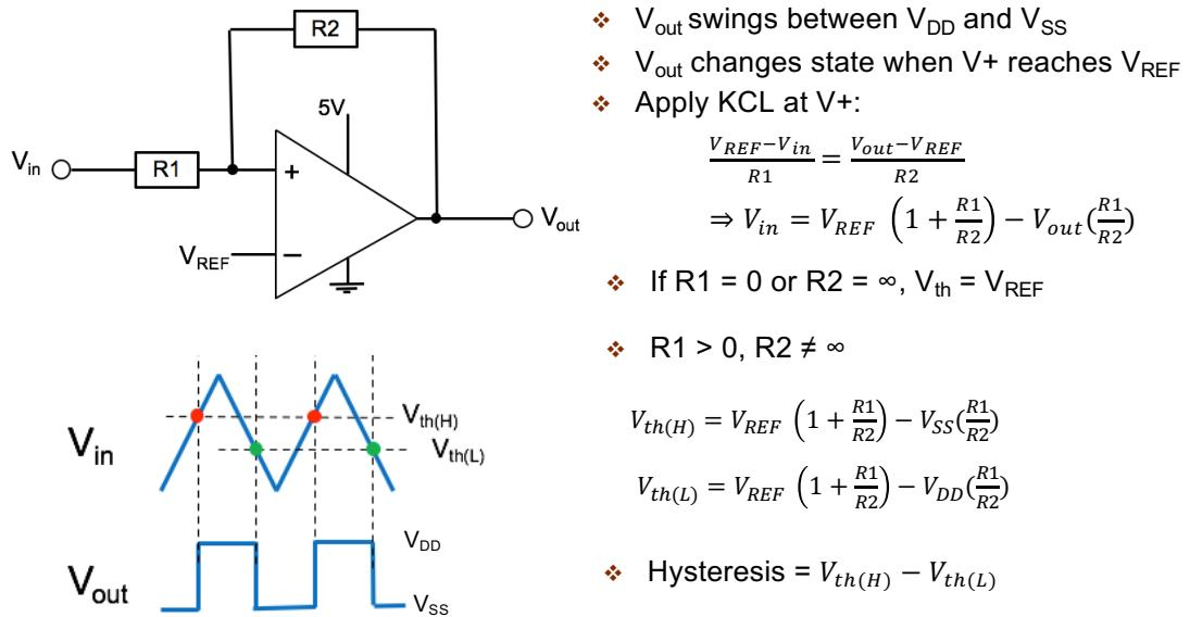
Op-amp can be used as an analogue comparator. In the circuit shown, V<sub>REF</sub> is constant voltage that defines the comparator threshold for switching output from high (V<sub>DD</sub>) to low (V<sub>SS</sub>) voltages. V<sub>out</sub> changes state when V<sub>+</sub> reaches V<sub>REF</sub> from either direction (i.e. with V<sub>in</sub> rising or falling).
