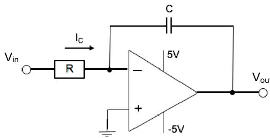
❖  $v_{out} = -\frac{V_{in}}{RC} t + V_C(0)$
